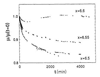
Figure 3: Time dependence at room temperature after Ar ion laser light illumination at 77 K of the mobility  $\mu$  for YBCO films of different oxygen content  $x_n$ . Values have been normalised to the initial value, which for all samples is  $4.2 \pm 0.3 \text{ cm}^2/\text{V.sec.}$
