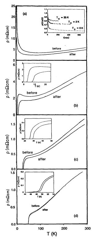
Figure 1: Electrical resistivity vs temperature before and immediately after laser illumination for YBCO films with nominal oxygen stoichiometries (a)  $x_n = 6.5$ , (b)  $x_n = 6.55$ , (c)  $x_n = 6.6$  and (d)  $x_n = 6.6$ . The inset in (a) shows the time evolution of the resistivity at 77 K during illumination for samples a, b and c. The insets in (b), (c) and (d) show the region near  $T_c$  in expanded scale.
