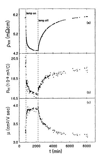
Figure 2: Time dependence at room temperature during and after halogen white light illumination of (a) the electrical resistivity  $\rho$ , (b) Hall coefficient  $R_H$ , and (c) mobility  $\mu$ , for an  $x_n = 6.5$  YBCO film.
