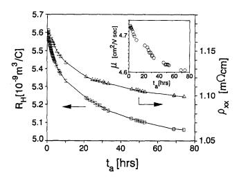
Figure 4: Time dependence at room temperature, starting immediately after deoxygenation, of the electrical resistivity  $\rho$ , and Hall coefficient  $R_H$ , for a non-illuminated  $x_n = 6.6$  YBCO film. Inset shows the time dependence of the mobility  $\mu$ . Solid lines are guides to the eye.
